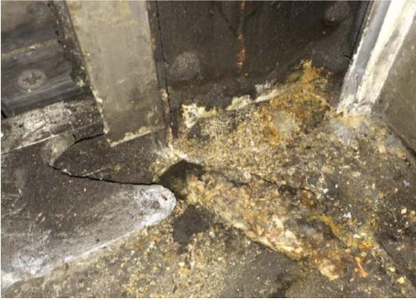
7 Internal door pillar corrosion
