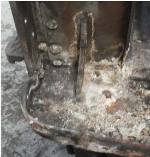
3 Car body corner post corrosion
