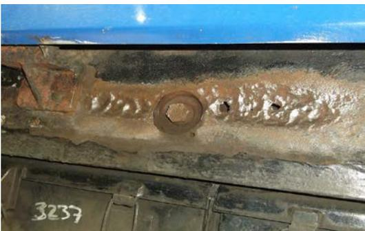
5 New sole bar holes and corrosion
