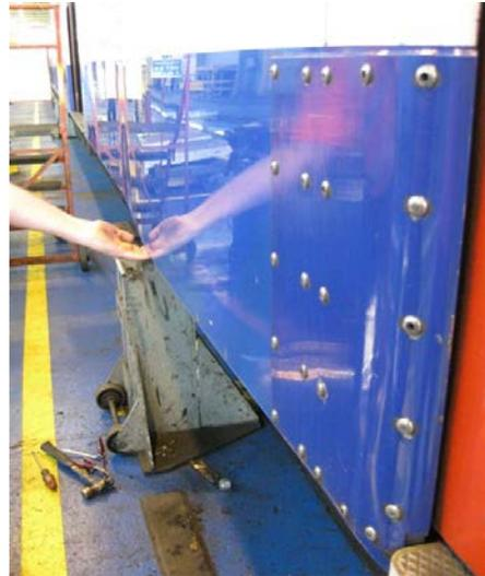
10 Failed car body side stiffener bracket
