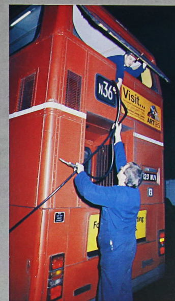
Simon Kelly (top) and Peter Mould top up a header tank with water during their night shift at Peckham Bus Garage
